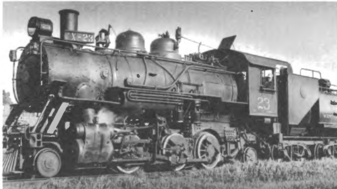
CWR Engine #23, one of the three 2-6-2 sister engines built by Baldwin. She was purchased in 1923 and scrapped in 1950.
