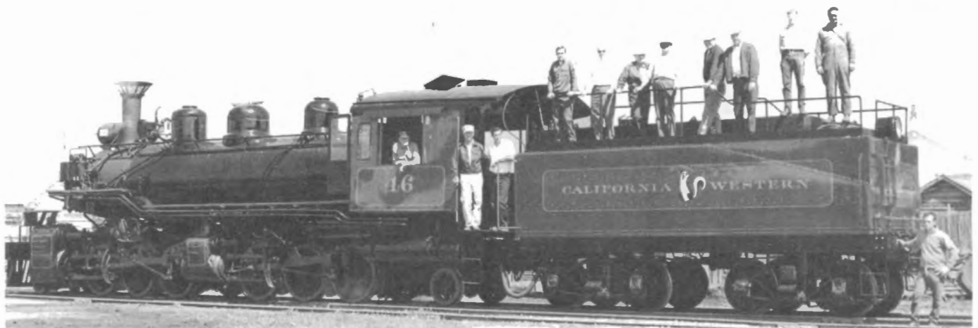
The California Western shop crew stands on the tender behind Engine #46, after the restoration in 1970. The Mallet was built by Baldwin as a saddle tank engine without a tender.
