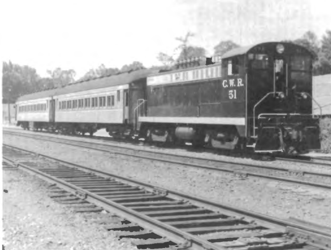
California Western Railroad's first diesel electric locomotive, Engine #51, Baldwin Locomotive Works C/N 74408, a 750 HP unit built in 1949, sits in the Willits yard with a passenger consist.
